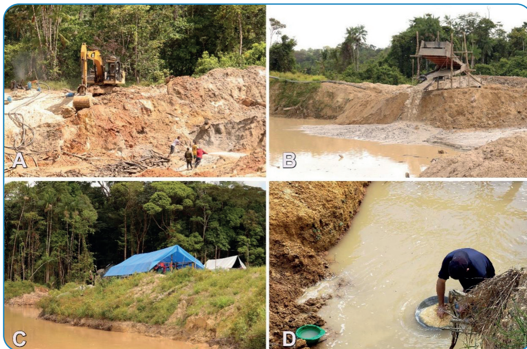
FIGURE 1: Illegal mining activities in the Brazilian Amazon region, Garimpo do Lourenço, Calçoene-Amapá. The images show mining activities in the Brazilian Amazon region, displaying an excavator ( A ), a washing equipment (also known as Curimã) ( B ), a housing structure ( C ), and artisanal mining utilizing a tray (also known as bateia) ( D ). Photos by MORESCO, G and AMARAL, PST.
